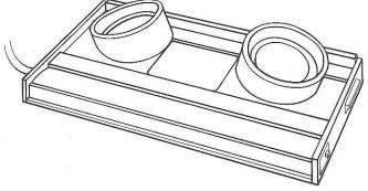
The acoustic coupler is a box with two foam rubber rings on it and a cable coming out. The handset of your phone plugs into the rubber rings, and the cable plugs into your modem. With that done, you're all set.
