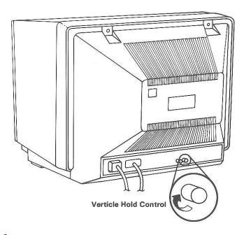
Turn the Vertical Hold control counterclockwise until the screen stops rolling and is stable.
