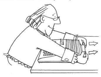
forming a groove or slot at the front edge of the lid. Put the front of the lid down onto the main unit so that the lip of the case just above the keyboard slips into that groove or slot. Center the lid, lining it up with the bottom piece of the case, and then press the back of the lid down firmly. The two latches should snap into the indentations on the rear of the lid.
