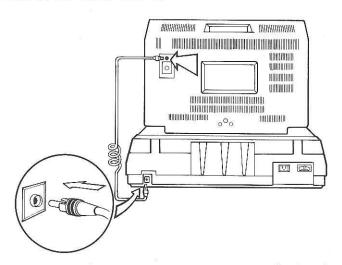
The other end of the cable connects to your display device. If you're using a video monitor, the cable plugs right into a female connector similar to the one at the back of the ACE. If you're
